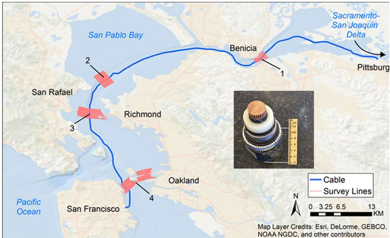
Figure 2-1 The Trans Bay Cable route (thick blue line) from Pittsburg, CA (upper right) to San Francisco, CA (lower left) showing locations of magnetometer surveys (red lines):
